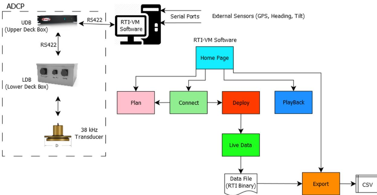
Figure 20. RTI Vessel Mount Functional Diagram
