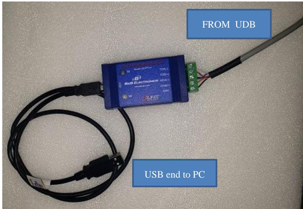
Figure 10. Showing the Blue communication terminal block that connects the Communication cable from the Upper deck box and the PC. The USB end of the terminal block gets plugged into the PC to establish the connection between the Ship PC and ADCP.
