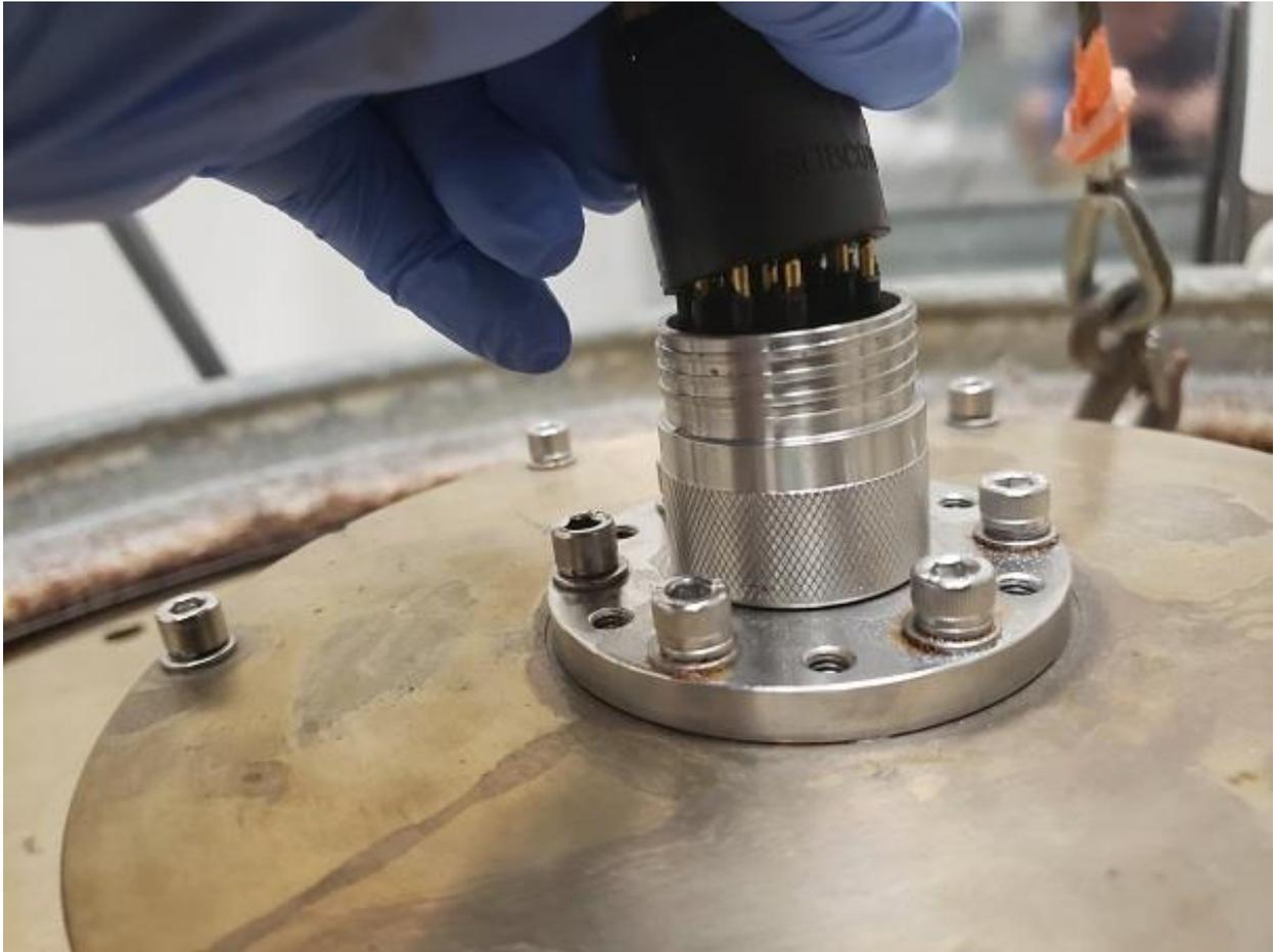
**Figure 13:** shows the transducer cable inserted into the female connector on the transducer endcap.
