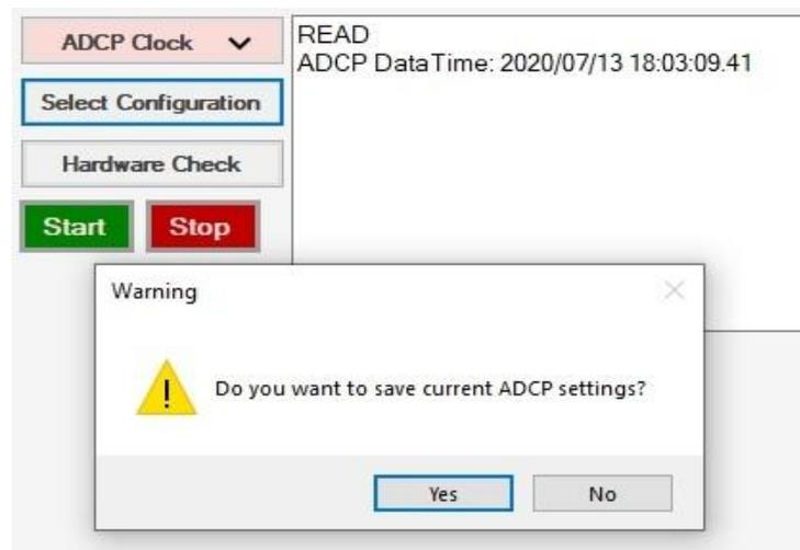
Figure 32. Option to save current ADCP configuration
