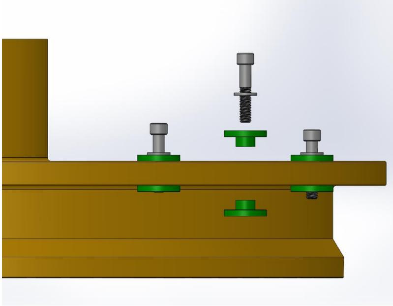
**Figure 16. Side view of the illustration of the isolators used in the VM unit on top and bottom side.**
