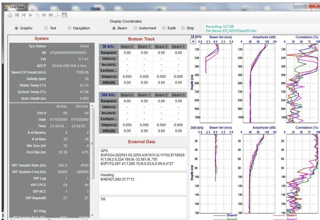
Figure 38. Live Data Display showing a 38/300 kHz dual frequency system data
