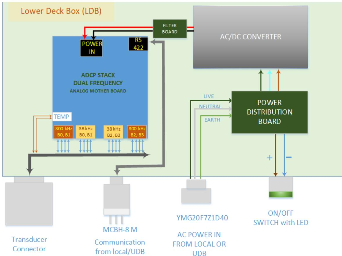
**Figure 5. Internal block diagram of the Lower deck box showing the connections between the various interfaces. LDB is the lower deck box and UDB is the upper deck box.**
