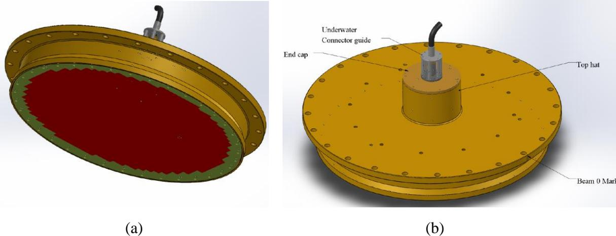
Figure 7 . Vessel Mount Dual-Frequency transducer housing showing the (a) transducer face encapsulated with red colored poly urethane and (b) the top view showing the underwater connector guide, top hat, Beam 0 Mark.
