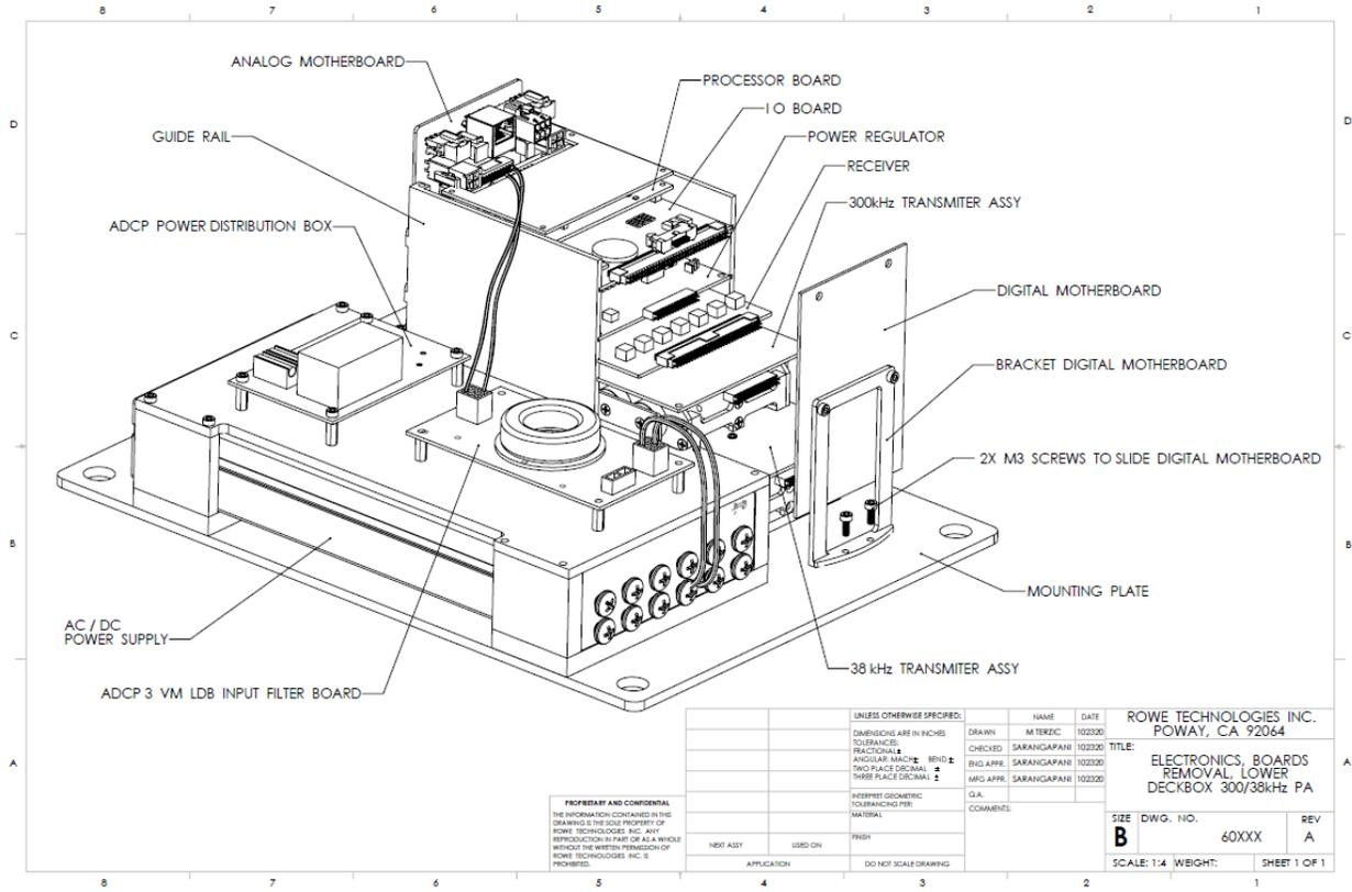
**Figure 50 Mechanical drawing showing all the components of the electronics stack inside the Lower Deck Box.**
