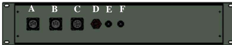
**Figure 4. Back view of the Upper deck unit with labels showing the various connectors. A) AC power in from Ship, B) AC Power to Lower Deck Box (LDB), C) Communication from Ship PC, D) Communication cable to Lower Deck Box (LDB), E) Trigger in, F) Trigger out.**
