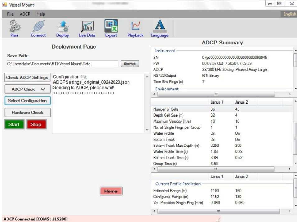
Figure 33. Sending configuration to ADCP
