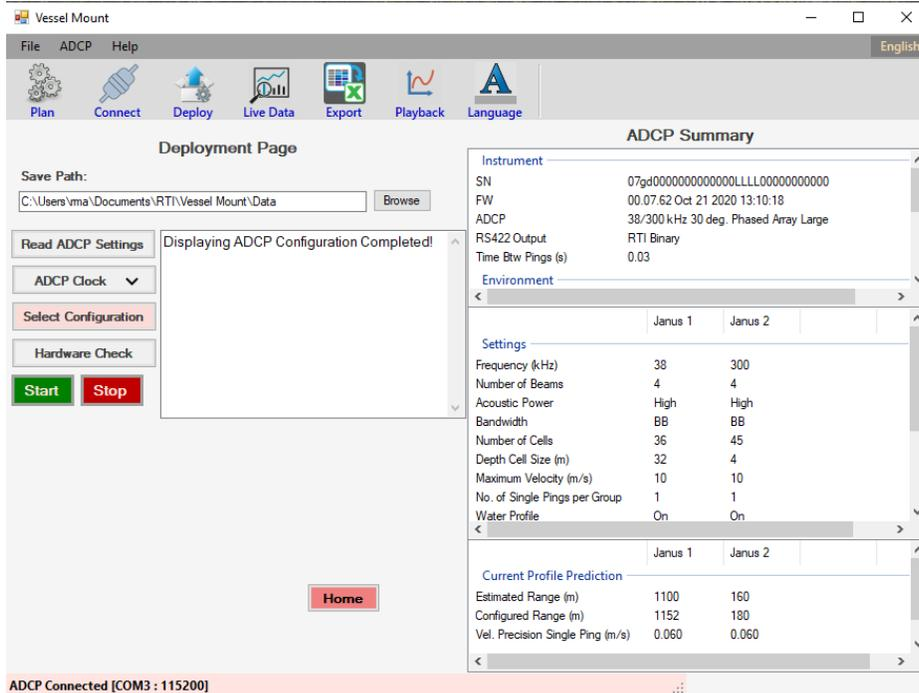
Figure 34. Read back ADCP configuration after it was sent to ADCP
