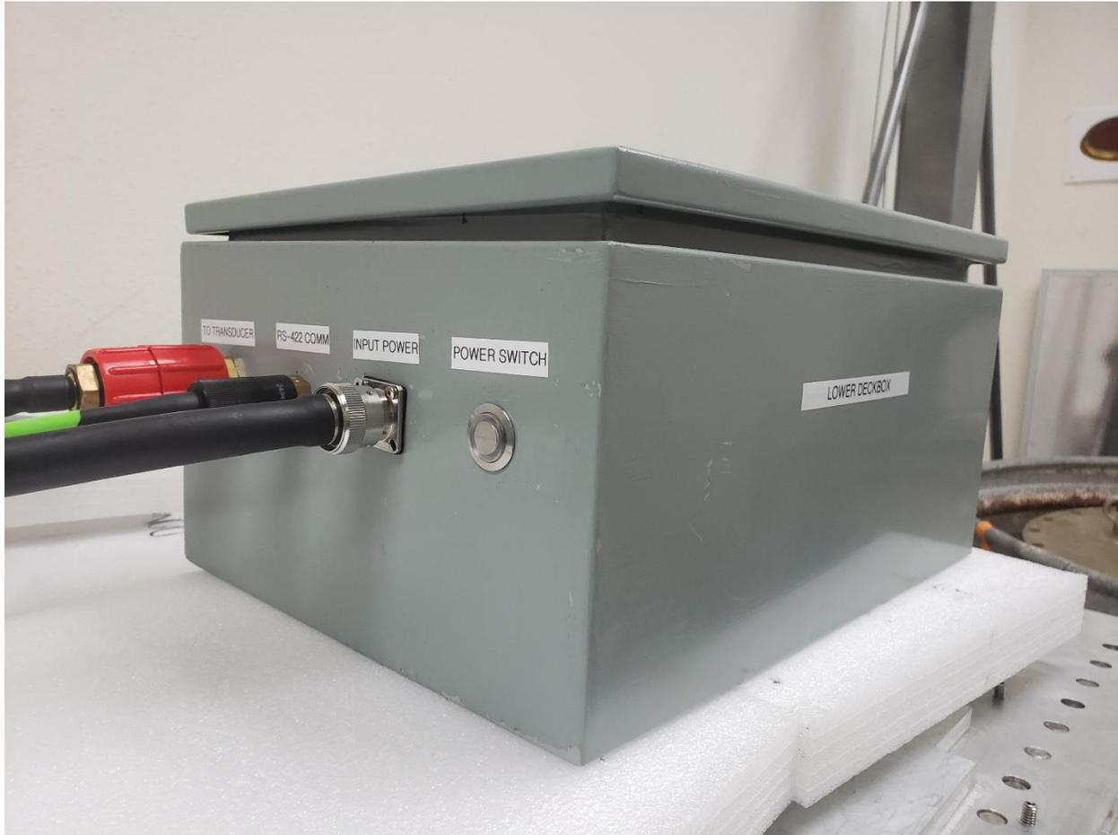
**Figure 12:** This picture shows the cables connected to the Lower Deck Box. The Power Switch is also shown.
