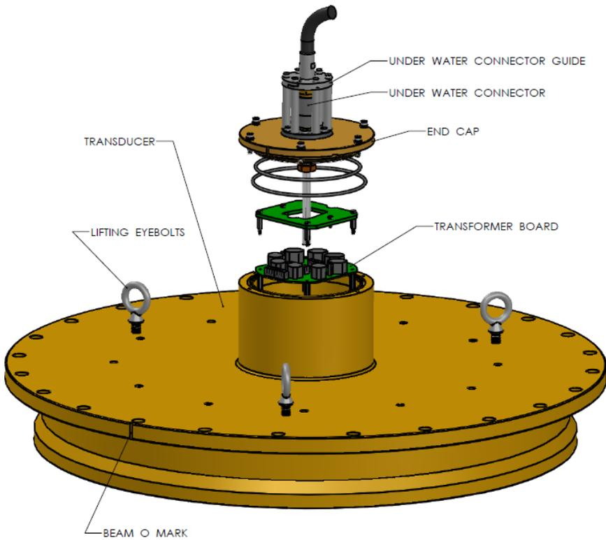
Figure 8. Side view of the Dual Frequency VM transducer in bronze housing with eyebolts used for lifting the transducer and exploded view of the transformer board in the transducer housing. The underwater connector guide (Carriage), underwater connector in the end cap is also shown.
