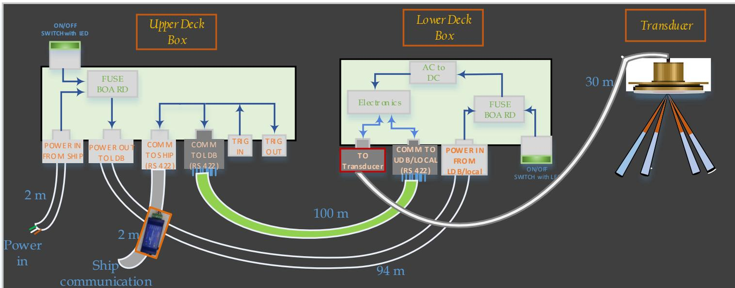
Figure 17. System Block diagram with Interconnections showing the different blocks and connections in the VM-DF ADCP system.
