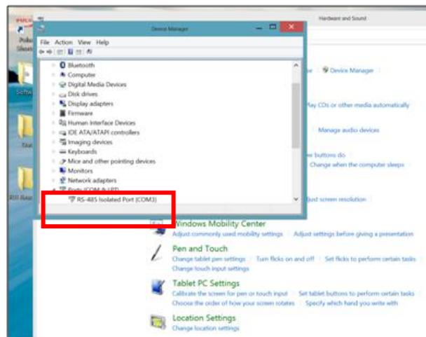
Figure 18. RS 485 Isolated COM Port setup.
