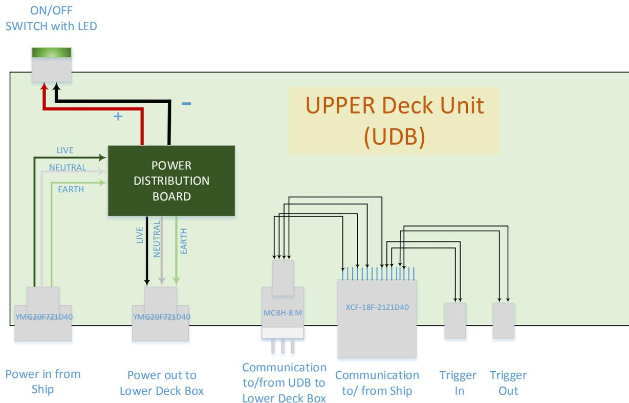
**Figure 2. Internal block diagram of the upper deck unit showing the connections between the various connectors. LDB is the lower deck box and UDB is the upper deck box.**
