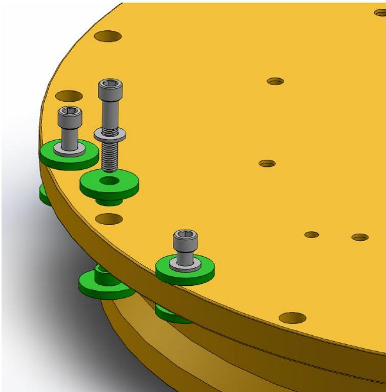
**Figure 15. Illustration of the mechanical isolators (green) used in the VM unit. The purpose of the isolators is to isolate or reduce the noise coupling to the transducer.**
