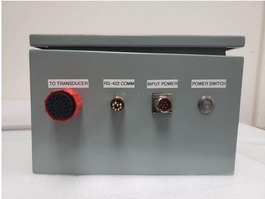
Figure 11: Side View of the Lower Deck Box showing the Transducer Connector, RS-422 Communication to Upper deck box/local PC, power input from the Upper Deck Box/ Local, input power, Power Switch with LED.
