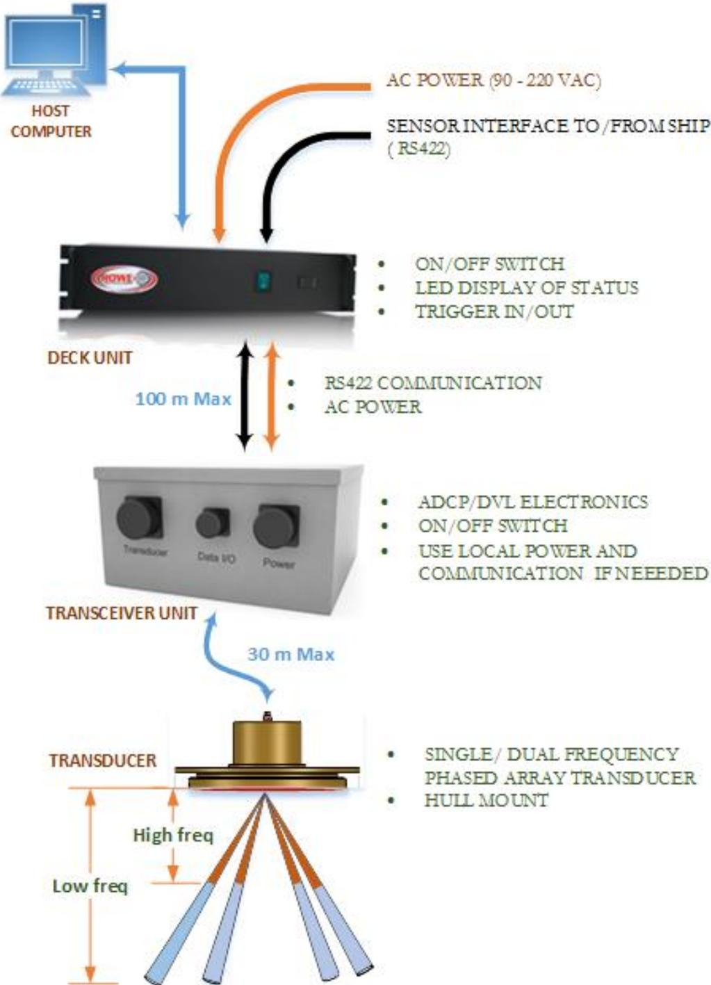
Figure 1. System block diagram of the Sea Surveyor VM 38/300 kHz. The high frequency beams (300 kHz) is denoted in orange and the low frequency beams (38 kHz) is denoted by blue from the transducer.
