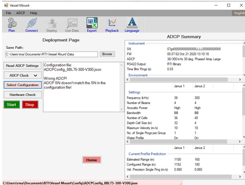
Figure 35. Sending a configuration to a wrong ADCP
